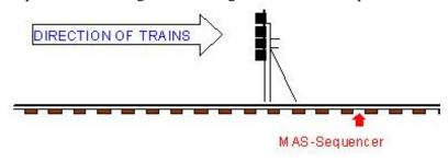
The MAS-Sequencer can be used on its own to control a single signal. If more than one signal is on the same line the extra signals can be operated by IRDASC-4 units. A connection from the MAS-Sequencer s "send" terminal to the following IRDASC-4s "receive" terminal tells the IRDASC-4 which aspect the MAS-
