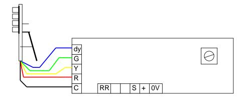
The diagram shows a 4 aspect common negative signal (all the short legs, cathodes, of the LEDs connect to the C Terminal).
