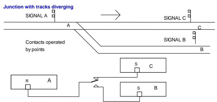
A changeover contact operated by the points movement is required. This feeds IRDASC A with the send "S" of whichever IRDASC the route is set for.
