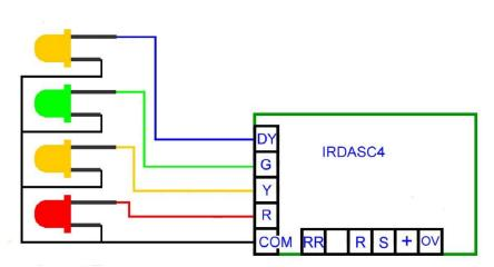
negative or common positive wiring. C=common R=red Y=yellow DY=double yellow (extra yellow for 4 aspect signal) G=green
